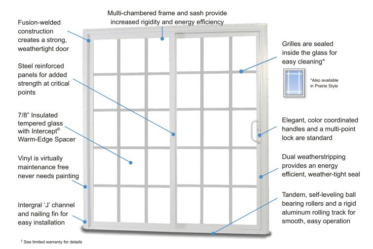
**Built to Last:** The series 5800 is designed and built to provide a lifetime of reliable performance. It features a wider, thicker profile for added strength and a more traditional appearance. Fusion-welded construction creates a strong, weather-tight door.
