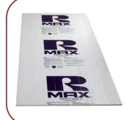
R-Matte<sup>®</sup> Plus-3 is a rigid foam plastic thermal insulation board composed of environmentally sound, closed cell, polyisocyanurate foam bonded to a durable white-matte (non-glare) aluminum facer and a reflective reinforced aluminum facer.
